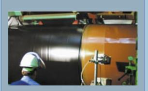
**Serie FP** series is based on fusion bond epoxy which provides excellent protection against corrosion. FP series coatings meet all pipeline specifications.
